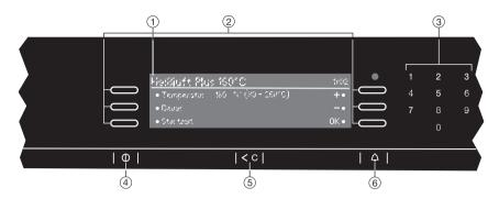
The appliance is operated via the display 1 and the electronic sensors next to and below the display. These react to finger contact. A keypad tone will sound each time a sensor is touched. The volume of the keypad tone can be adjusted or switched off altogether (see "Settings - Volume - Keypad tone").
